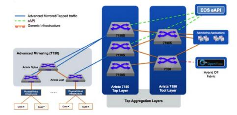
Both of the above approaches leverage the onboard advanced monitoring feature set enabling the capture and analysis endpoints to receive the specific data of interest in the format expected.
